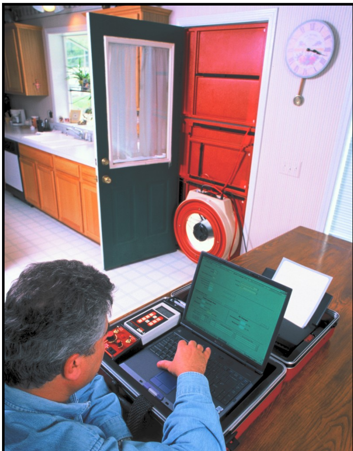
The Infiltrator test pinpoints air leaks in your house and duct system
